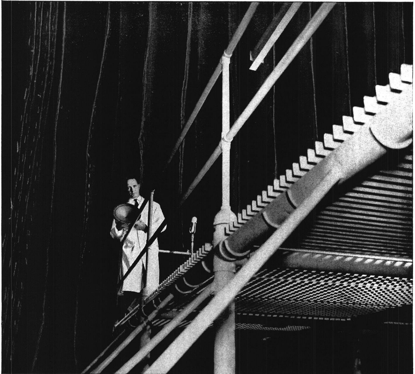
At David Sarnoff Research Center, Princeton, N. J., RCA tests one of loudspeakers used in new high fidelity "Victrola" phonographs.
