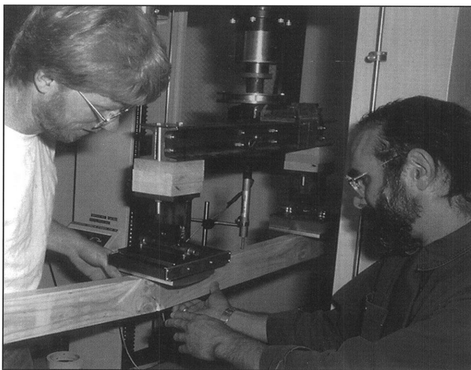
Improving utilisation of forest resources: mechanical testing of lumber cut from small-diameter timber.
