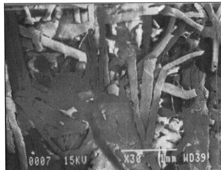
Scanning electron micrograph of hot-pressed agricultural fiber that has been modified to have thermoplastic properties. For comparison, the photo on the right is unmodified fiber.
