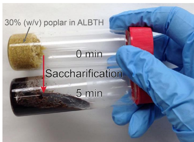
Figure S4.1 Liquefaction of poplar at 30% (w/v) loading in ALBTH at 110 °C for 5 min.
