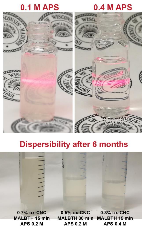
Figure S6.7 Pictures of ox-CNC suspensions showing the Tyndall effect with laser light passing through (A) and the colloidal stability after 6 month (B).
