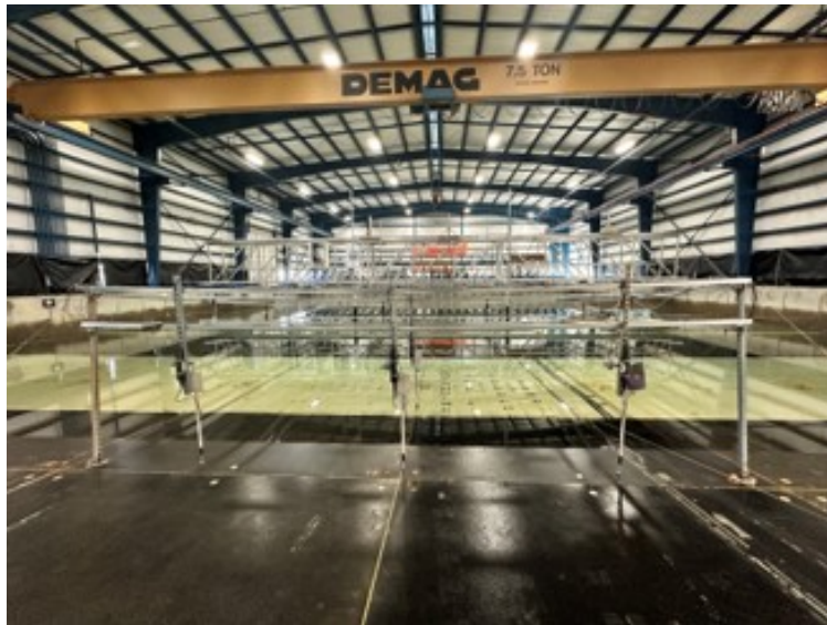
Figure 4.1: Image of the instrument arrangement in the directional wave basin.
