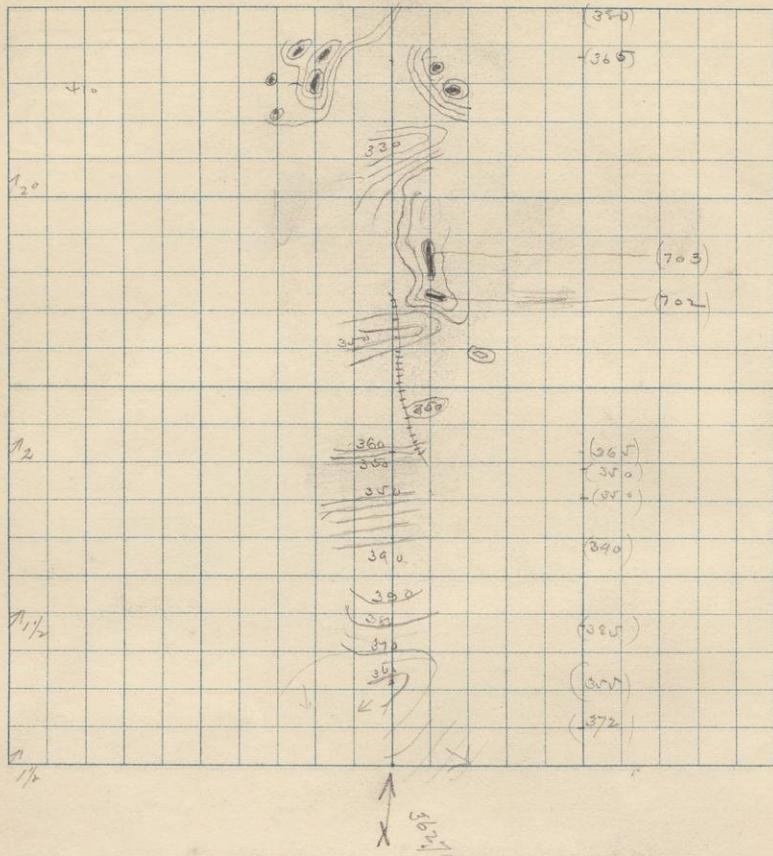
The four succeeding contour sketches show approximately the character of secs 32 x 29 - 43 - 31. The surface is almost one mass of rocks with knolls & cliffs as storm. It was impossible to get correct contouring with only four guns through the seas and
