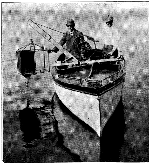
Fig. 2. Plankton trap and equipment for operating it.
