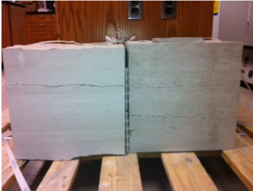
Figure 2. Photo of fractured dolomite samples obtained from the quarry. The horizontal fractures are clear from this photo. Smaller horizontal fractures that are not readily observable in the photos are also present.
