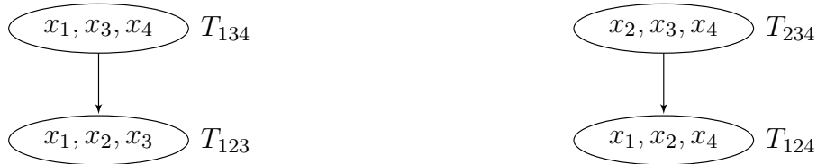
Figure 2.2: Two rooted tree decompositions for the 4-cycle query (Example 2.3). Annotations such as T_{123} denote the intermediate join results at the corresponding bags, e.g. T_{123} = R_{12} \bowtie R_{23} .
