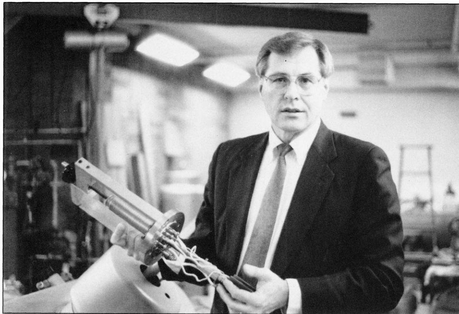
Kulcinski holds one of the many "tools of the trade," a proton accelerator used to test the resistance of materials to radiation damage.
