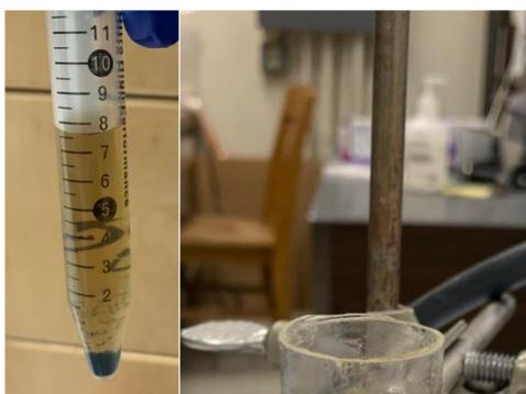
**Figure D.S10.** Photographs of the methylarene oxidation reaction solution without (left) and with (right) 20 mM NiNO<sub>3</sub> and the RR as the counter electrode. A dark blue precipitate was present if NiNO<sub>3</sub> was not added to stabilize the NiHCF crystal structure.
