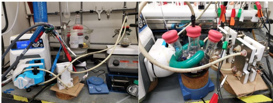
**Figure 2A.4.** Graphic illustration of the undivided flow cell for 12 mmol (left) and 48 mmol (right) scale-up.
