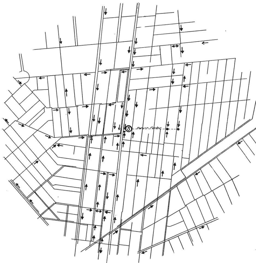
FIG. 5.—Typical Current Survey Plotted on Skeleton Map of Section of City Showing Underground Mains and Stray Currents Flowing on Mains.
