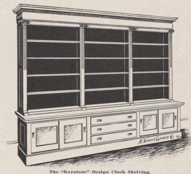
Minimum length, 12'. Made any lengths to order. Standard height of base to match wall cases, 2' 6" high, 2' deep. Upper parts same height as wall cases. Shelves 10" wide. The "Dixon" design has beveled plate mirror of suitable design to set in recess as shown. Made any dimensions.
