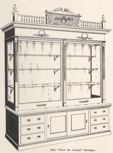
Made any length. Height of base 30"; width of base, 30"; height of top part, 60" inside; top part is 14" deep inside. Upper doors slide up, lower doors slide sideways. DSAa glass. Felt covered wood shelves on brackets. Backs are lined with black cloth, top and bottom painted. Upper part knock-down. Best in finish, A No. 1 construction. Ball-bearing, counterbalanced, dust-proof doors. Good hardwood shelves on adjustable brackets, mirror backs, plate glass shelves, etc., at additional cost.
