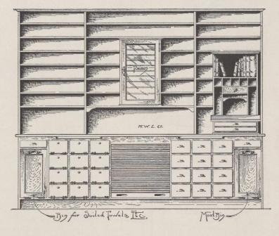
No. 304. It is the "Druggist's Ideal." Has bottle cubbies, cork drawers, tool drawers, meal and soiled towel bins that tilt, pill slides, cupboards for mortars and graduates, with roll curtains in place of door, thus being out of the way, open or closed; has poison case, pigeon hole case, label desk, adjustable shelves and hard maple top.
