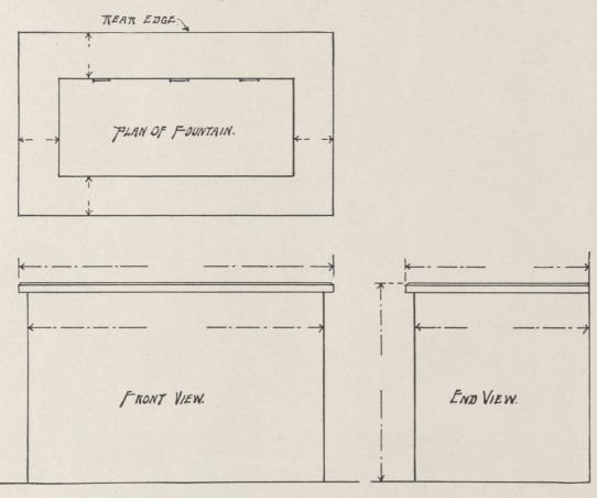
The above cuts illustrate the top, the front and the end of a soda fountain apparatus, the dotted lines show the measurements we would require. Make a rough pencil sketch of your fountain, showing top, front and end views as above and mark in the necessary measurements
