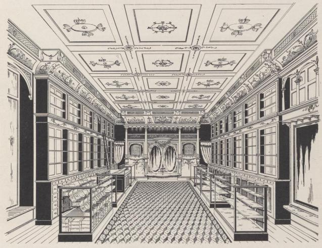
Sketch shows a complete interior of a double decker with sliding ladders. Notice the prescription cross partition with columns supporting ceiling, oval mirrors and recesses. Cases used are the "Cornwell" floor cases with straight down wood base.
