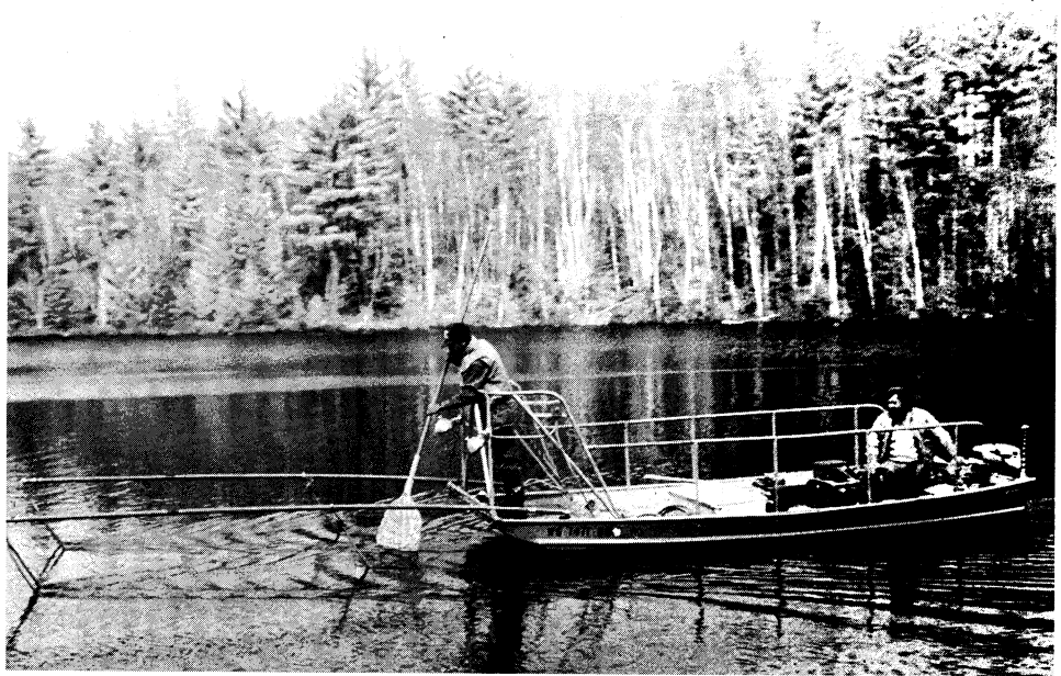
AC-electrofishing gear used to sample fall fingerling smallmouth bass. Sandy Engel, left, and Gary R. Kubenik, right.
