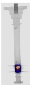
Figure 5.14 PET/CT image of ^{68}\text{Ge}/^{68}\text{Ga} trapped in a column filled with 245 mg \text{ZrO}_2 sorbent. The high density of \text{ZrO}_2 at the bottom of the column is manifested as a dark region due to low transmission of the x-rays from the CT scanner. The bright white spot inside the \text{ZrO}_2 material demonstrates how ^{68}\text{Ge}/^{68}\text{Ga} is mostly trapped in the upper part of the column.
