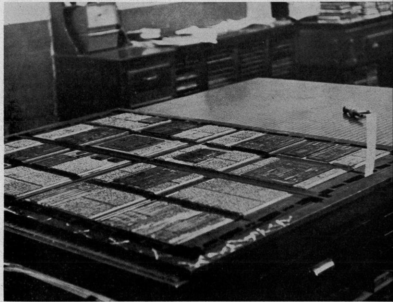
Engravings are mounted (top right), a proof of the completed page is then taken (above), and read for corrections, and then the pages are locked in proper sequence into a chase (right). The chase is then put on the press and made ready for printing. Below, Wally Ottum (left), plant superintendent, and Ted Olson, press room foreman, check a printed sheet for quality.
