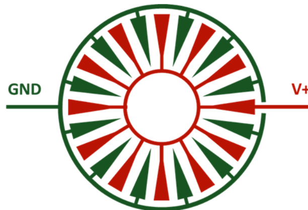
Figure 3.1. Schematic of areal density modulated electrodes used for electrowetting actuation. The interdigitated electrodes (+V) and counter electrodes (GND) cover an increasing percentage of the available area as the radius from center increases. This ensures that all forces on the oil droplet will be symmetric and that the droplet will be centered over the electrodes as voltage is applied.
