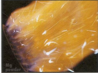
At right are flame tests of magnesium and zinc powders.
