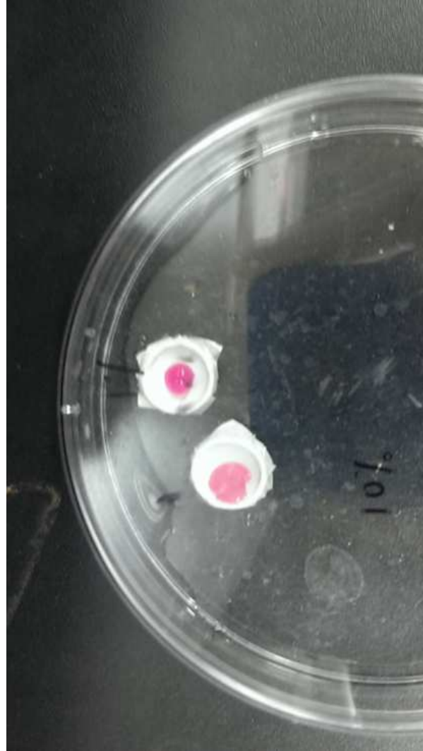
Figure 4.2: Droplets maintained for 24 hours at high humidity at 37 °C. Top droplet is DMEM + 1% FBS, while bottom droplet is DMEM + 10% FBS. The top droplet shows the spherical property expected from aqueous droplets on a superhydrophobic surface, while the bottom droplet shows degradation of the superhydrophobicity of the substrate
