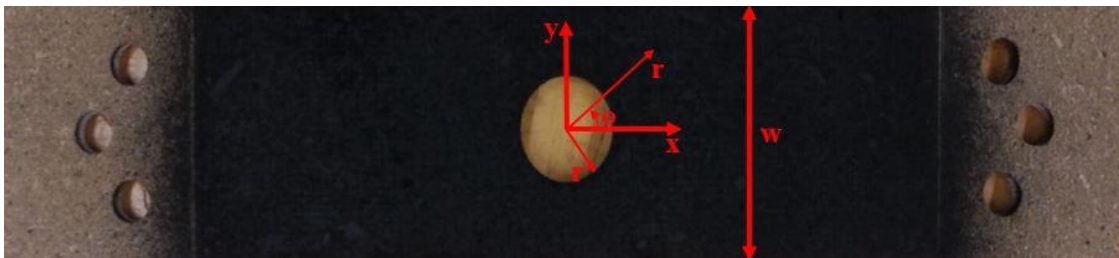
Figure 2.1.1: Black painted perforated cellulose-manure composite plate ( R = 12.7 mm, w = 62 mm, t = 7.2 mm)
