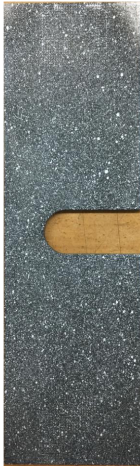
Figure 5.4.1: White speckle pattern applied on the plate for DIC
