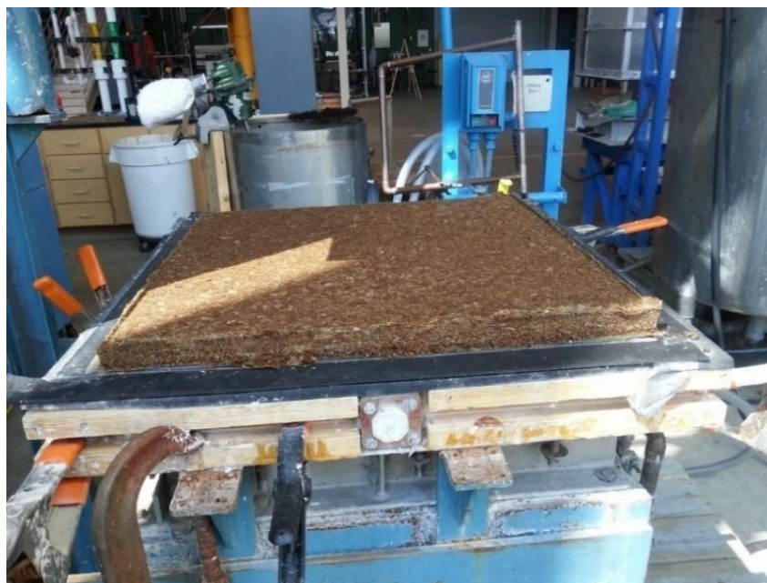
Figure 2.2.2: Wet-formed composite mat prior to the application of heat and pressure
