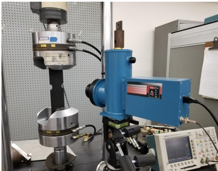
Figure 6.5.2: Recording thermal data in tensile loaded double-notched composite specimen with infrared camera
