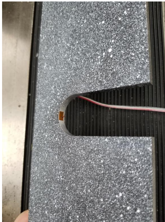
Figure 4.6.12: Strain gage location
