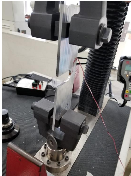
Figure 4.6.11: Strain gage mounted on notch at \theta = 180^\circ
