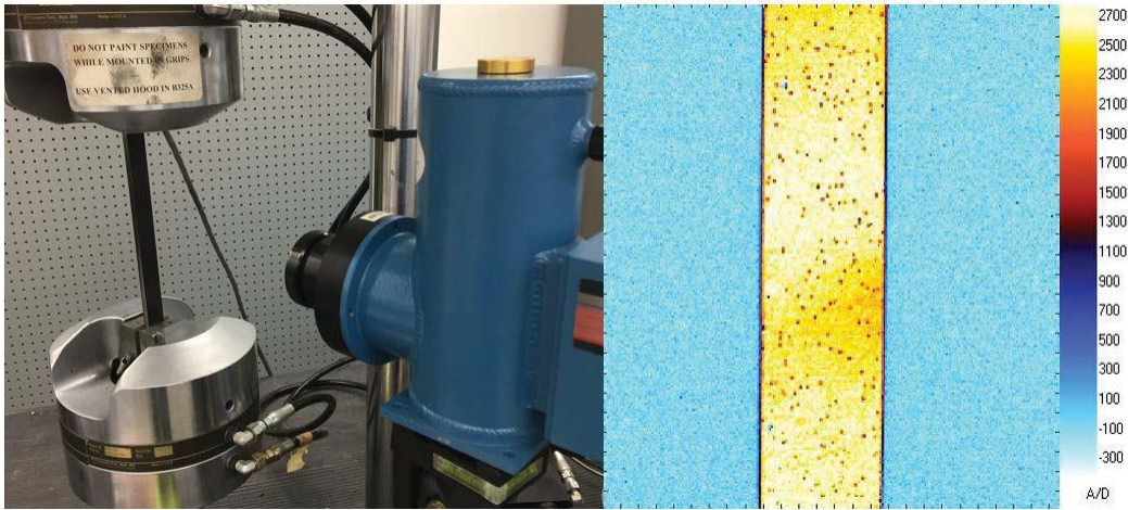
Figure 4.5.5: Experimental setup for uniaxial tensile aluminum coupon and TSA image
