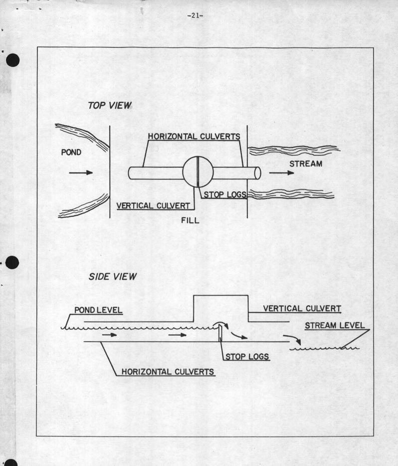
FIGURE 5. Drawing of outlet structure at Beaver Lodge Pond, Washburn County.
