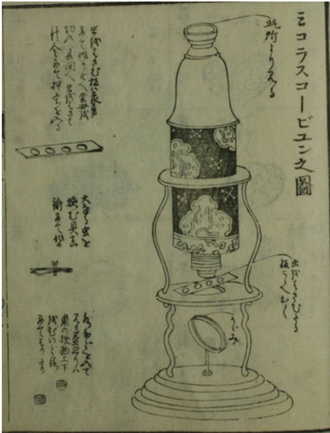
34 Illustration of a microscope from Morishima Chūryō's Random Tales of the Dutch . Detailed instructions teach the reader where to place samples and how to manipulate the instrument. Morishima Chūryō. Kōmō zatsuwa . 1787, Waseda University Libraries, Tokyo.
