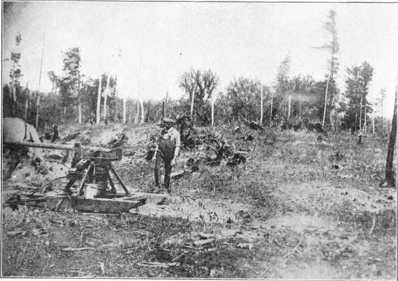
FIG. 1. A CHEAP BUT SATISFACTORY STUMP PULLER. The best results are obtained by supplementing its use with dynamite.
