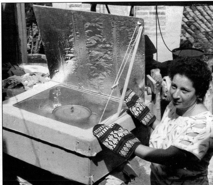
The solar box cooker will allow sun-rich but fuel-poor countries to take advantage of a free energy source and help prevent deforestation.
