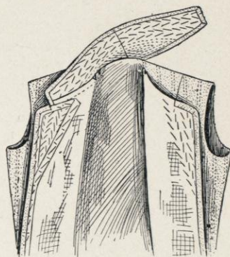
Fig. 307. Stretch the Collar Between Notches
