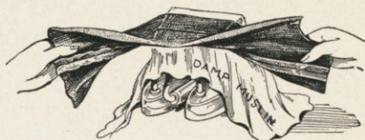
Fig. 325. The Proper Way to Open Seams in a Velvet Coat
