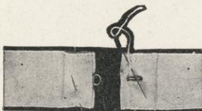
Fig. 240. Hook and Eye on Ends of Belt Tape
