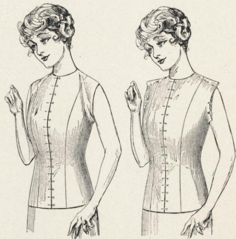
Fig. 197. Sloping Shoulders Make the Lining Wrinkle from Shoulder to Armhole
