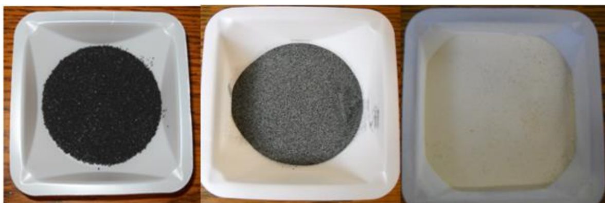
Figure 3.8. Picture of upper char+coke (>250 \mu\text{m} ), lower char+coke (<250 \mu\text{m} ), and the ZSM-5 catalyst after combustion of the char+coke.
