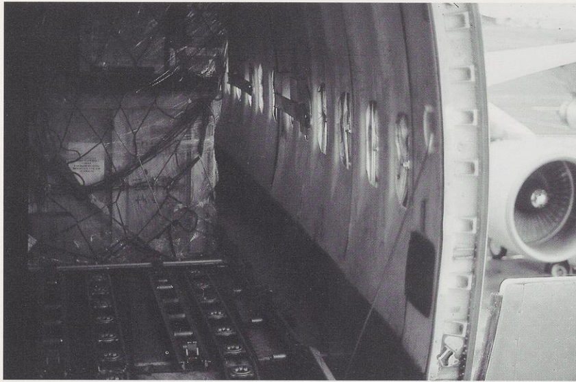
Pallets on the cargo deck, the floor equipped with rollers.
