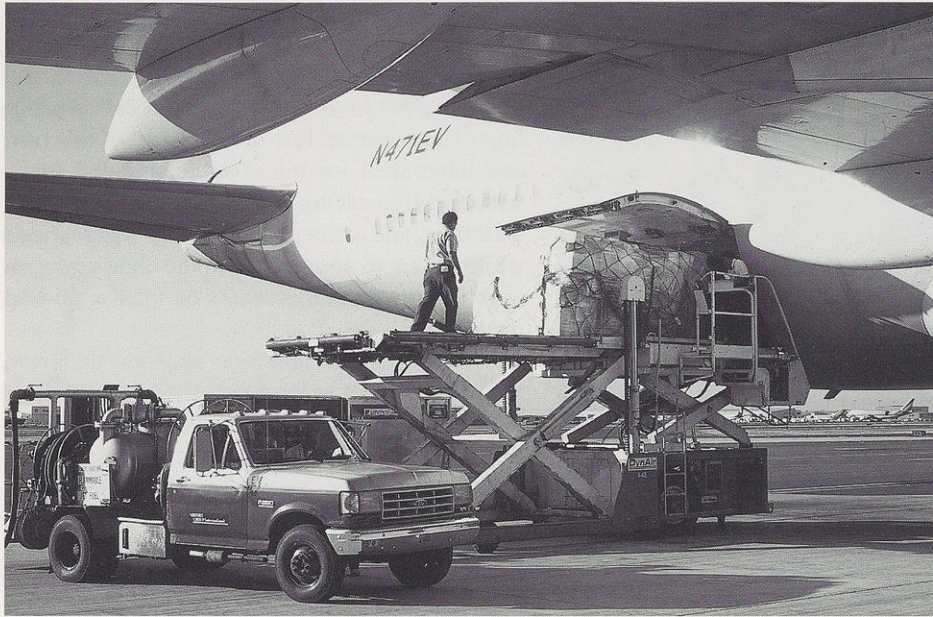
Pallets being loaded into the lower cargo deck of the Boeing 747 at Honolulu.
