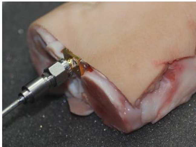
Figure 4.8. Measurement setup for the antenna under the skin.
