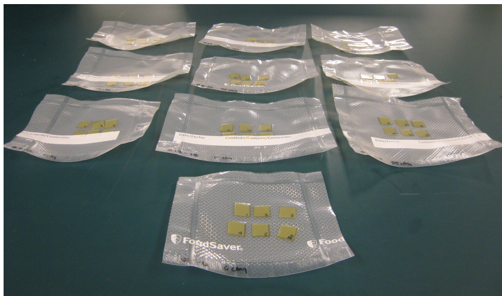
Figure 3.5: Photograph of film samples that were cut and placed in vacuum-sealed, air-tight bags using a commercially available food vacuum sealer.
