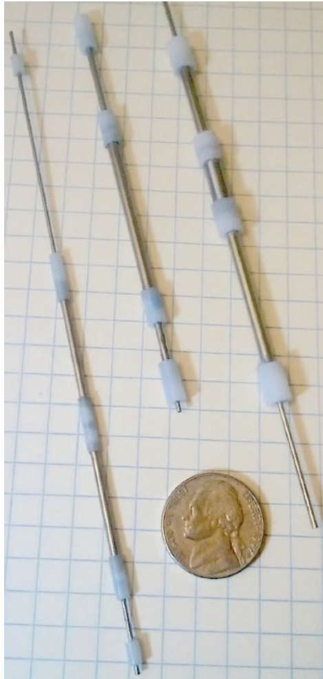
Figure 2.2: Photograph of the optimized needle inserts for 4 mm, 6 mm, and 8 mm cone collimators used by Bender (2014). For the 4 mm collimator, the optimized needle sizes are 15 and 20 gauge, for the 6 mm collimator the optimized sizes are 12, 16, and 20 gauge, and for the 8 mm collimator, the optimized sizes are 8, 12, and 18 gauge. Four machined plastic spacers are used on each assembly to allow concentric placement of the needles within the lead collimator. Reprinted with permission from E. T. Bender, “Increasing dose gradient and uniformity in small fields using modulation: Theory and prototypes for cone-based stereotactic radiosurgery,” Medical Physics , 41, 051706, 2014. Copyright 2014, American Association of Physicists in Medicine.
