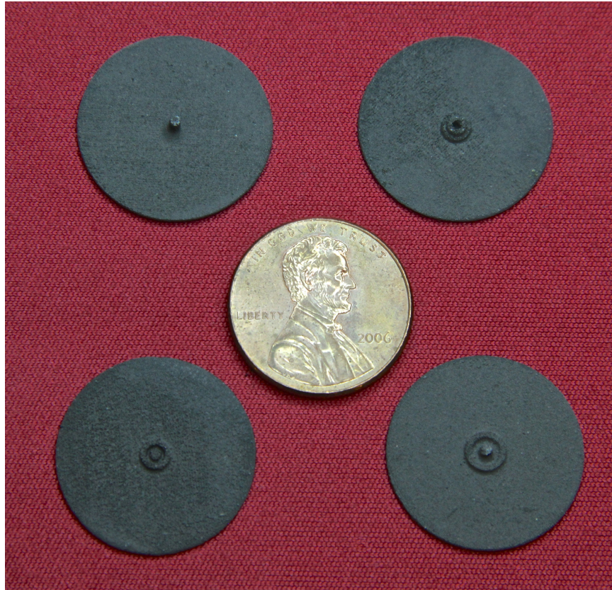
Figure 6.2: A photograph of the binderjetted epoxy-infiltrated bonded tungsten filter prototypes: 5 mm cone filter (upper left), 6 mm cone filter (upper right), 8 mm cone filter (lower left), and 10 mm cone filter (lower right).
