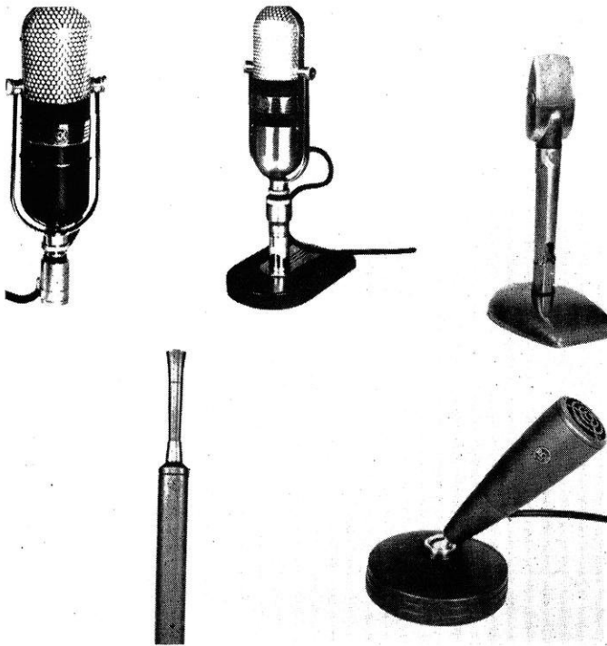
Pictured are five different RCA microphones showing design progress from 1938 to 1952. Top Row—Left: 1938, the RCA 77-C universal (ribbon type) microphone, a predecessor of the famous "77-D"; center: 1944, the popular RCA 77-D ribbon type, which may be used as a bi-directional, non-directional or uni-directional microphone; right: 1948, the RCA KB-2C "Bantam" velocity microphone, designed for studio or remote use. Bottom Row—Left: 1950, the RCA KB-4A "Starmaker" microphone, a ribbon-pressure type, designed especially for television use; right: 1952, the latest RCA microphone to be introduced is the BK-1A pressure type, successor to the "88-A".
