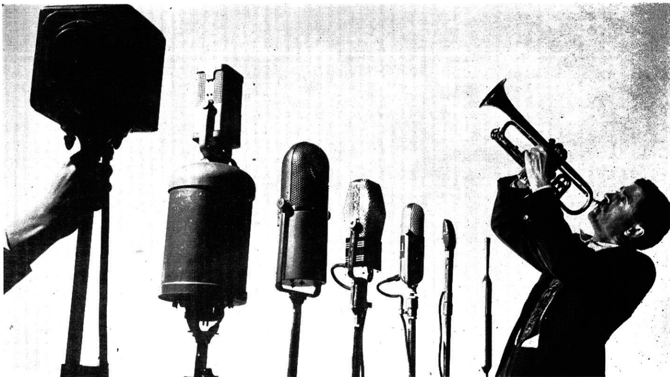
Musician hits a high note on his trumpet to test the performance of seven different microphones introduced by RCA since 1928. Microphones shown from left to right are: condenser type (1928), ribbon type (1930), universal ribbon type (1936), velocity type (1932), poly-directional ribbon type (1944), "Bantam" velocity type (1948), and the "Starmaker" ribbon pressure type.
