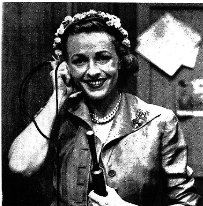
Robin Chandler is shown using an RCA "Starmaker" microphone during NBC's television coverage of the political conventions at Chicago. The "Starmaker," designed not to hide the faces of speakers or singers, is a non-directional, ribbon-pressure type microphone with a slender 7/8-inch diameter horn for increasing response in the high-frequency regions. It weighs only 15 ounces and handles equally all tones between 50 and 15,000 cycles.
