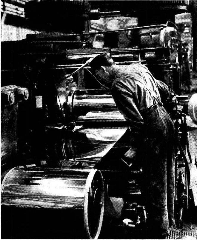
Above: A roll grinder is shown measuring the diameter of a work roll. The roll has been ground and polished to a mirror-like finish. The abrasive grinding wheel is back of the roll in the center of the photograph.
