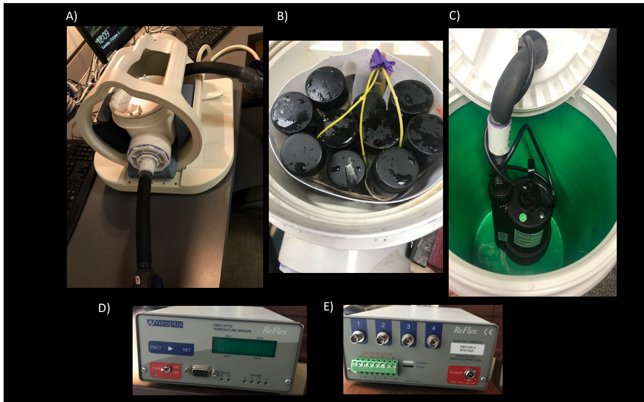
Figure 5.3 Temperature control system and monitoring. A) Backwater PVC valve used for housing the vials in the head coil for scanning, connected at two ends to high temperature hose for circulating water from and back to a reservoir in the control room. B) Vials with liquids in perforated plastic container placed inside the backwater valve; yellow fibers are the MR safe temperature probe leads for monitoring the temperature inside the housing. C) Sum pump used to circulate water through the backwater valve housing. D) and E) Digital reading system for temperature probe.
