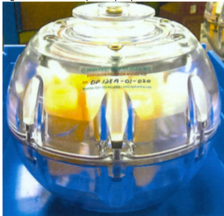
Figure 7. Assembled phantom. The top secondary fill port is closed by the pan head screw in the middle of the handle of the top fill port cap.
