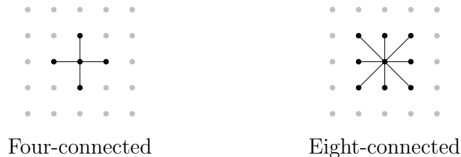
Figure 3.1: Illustration of neighborhoods of different connectivity, used to construct the graphs for MRF and Random Walker Segmentation. In the full graph, the highlighted neighborhoods will be repeated, centered on each grid vertex.
