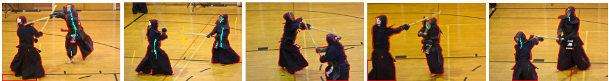
Figure 3.15: Interactive segmentation results using the multi-image model across five images from the “Kendo” set of iCoseg. As the number of images increases, less user input is required, as seen by the lack of such for the middle image.
