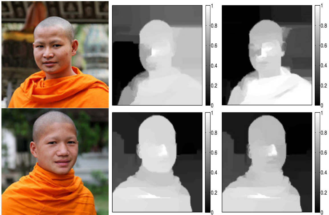
Figure 3.18: Effect of varying \lambda parameter on an example image for \lambda = 10^{-8} in Column 2, and \lambda = 10^{-6} in Column 3. A segmentation potential biased towards matching the histograms makes the partitions more pronounced.
