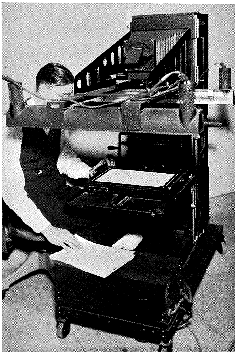
Copies of bank examinations made by the Banking Commission are furnished the banks. The photostat machine shown above reduces time and expense in making copies of these examinations.
