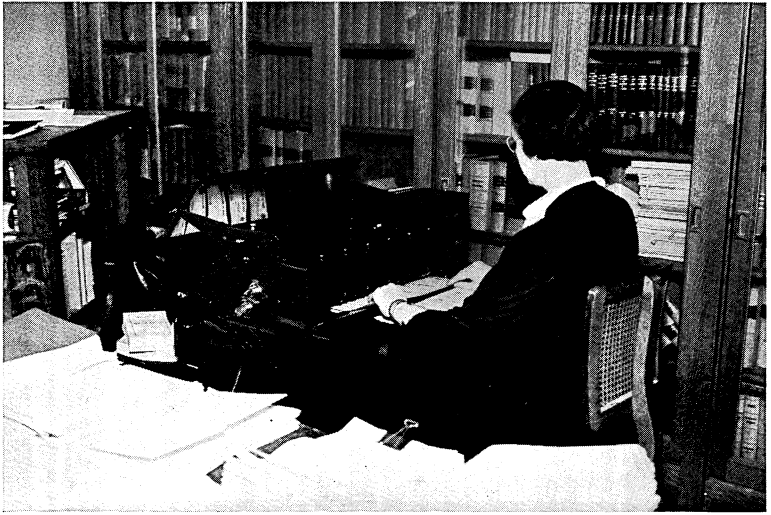
The electric check-signing machine in the State Treasurer's office. This machine writes the actual signature of the State Treasurer on the warrants.
