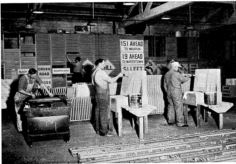
The State Highway Commission has a sign shop where directional signs to be placed on highways are made and painted.
