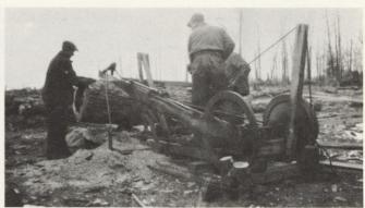
Logs cut with a "drag saw". One man rolled logs; another operated the saw rig; another took off the wood chunks on the John Nowicki farm.
