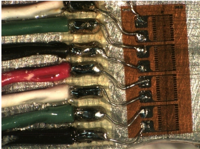
Fig. 8.90: Strip gage mounted along line CD of figure 8.1 and C'D' of figure 8.2
