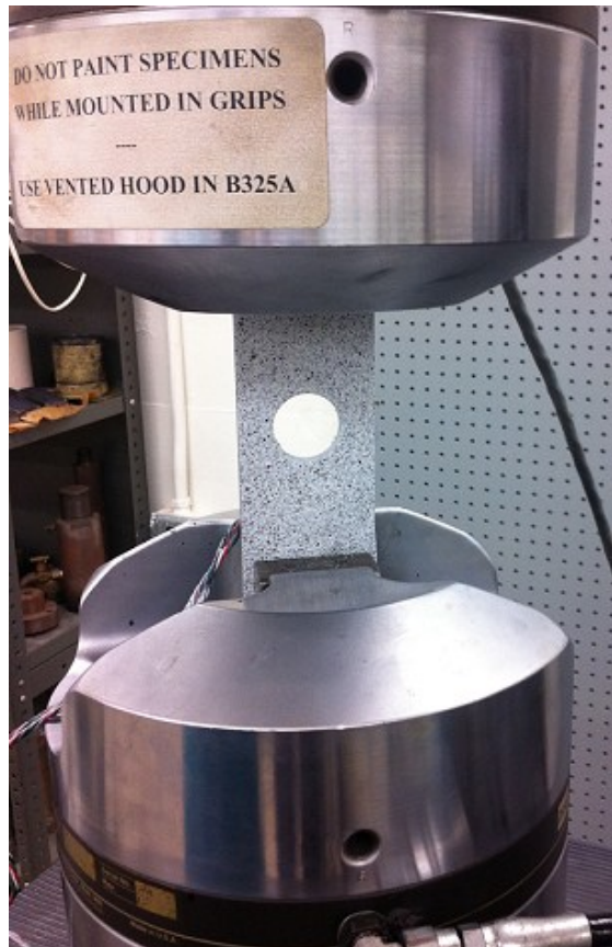
Fig. 2.23: Specimen loaded in hydraulic grips
