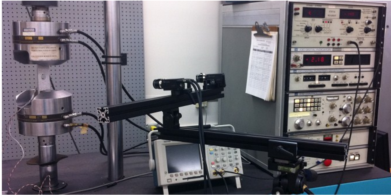
Fig. 2.24: Specimen loading and DIC recording
