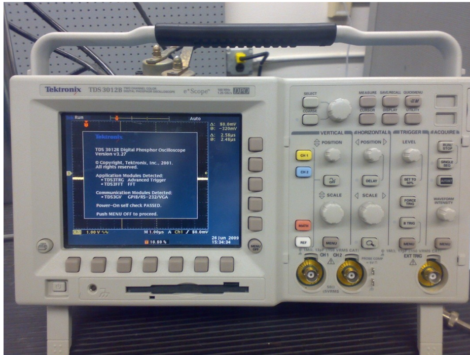
Fig. 8.8: Oscilloscope for accurate measurement of cyclic loads
