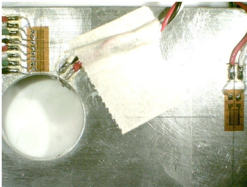
Fig. 8.91: Strip gage mounted along line CD and C'D' of figures 8.1 and 8.2 respectively, strain gage along the curved edge of the hole and the distant transverse strain gage
