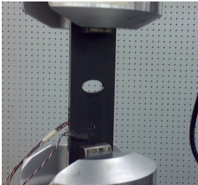
Fig. 5.7: Specimen loaded in hydraulic grips
