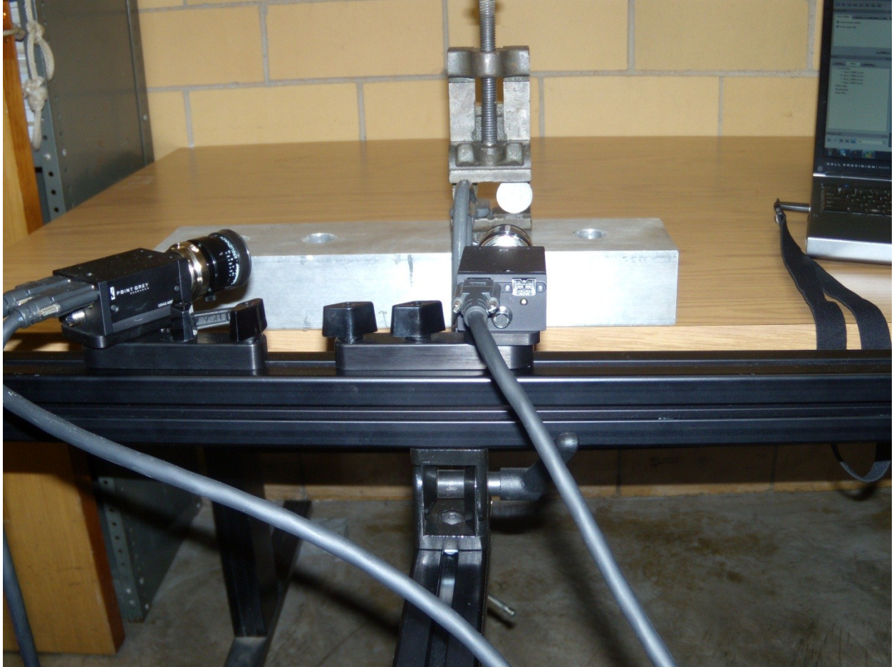
Fig. A2: Specimen in loading frame with DIC cameras
