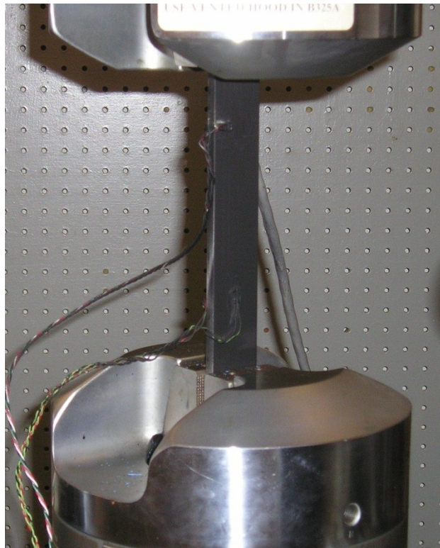
Fig. 8.14: Calibration specimen loaded in hydraulic grips
