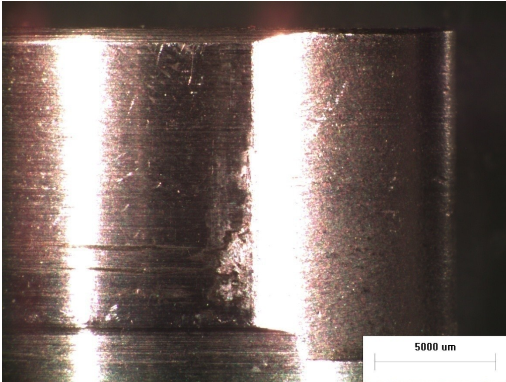
Fig. 6.39-B: Left boundary of the non-circular pin when facing the plate/pin from TSA side
