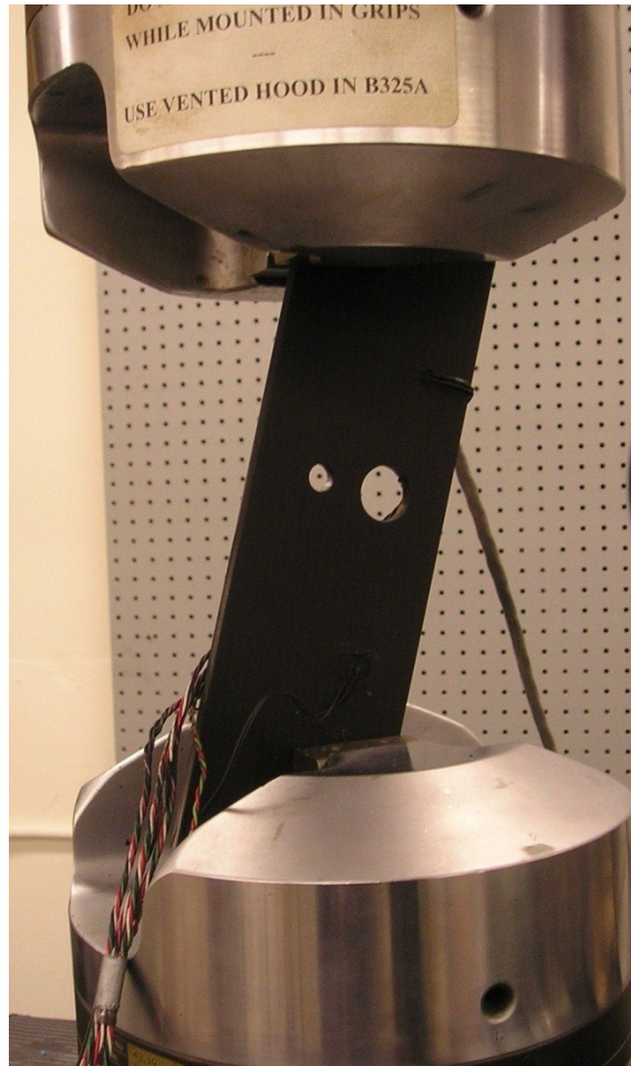
Fig. 8.5: Unsymmetrically-loaded specimen in hydraulic grips
