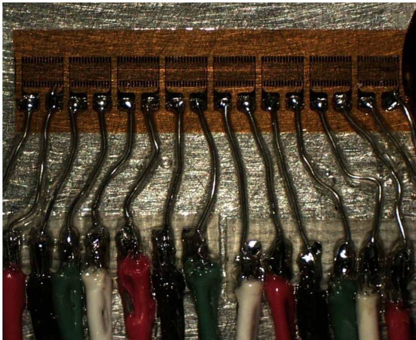
Fig. 5.41: Strip gage mounted along line AB of figure 5.2 (also seen in figures 5.38 and 5.40 )
