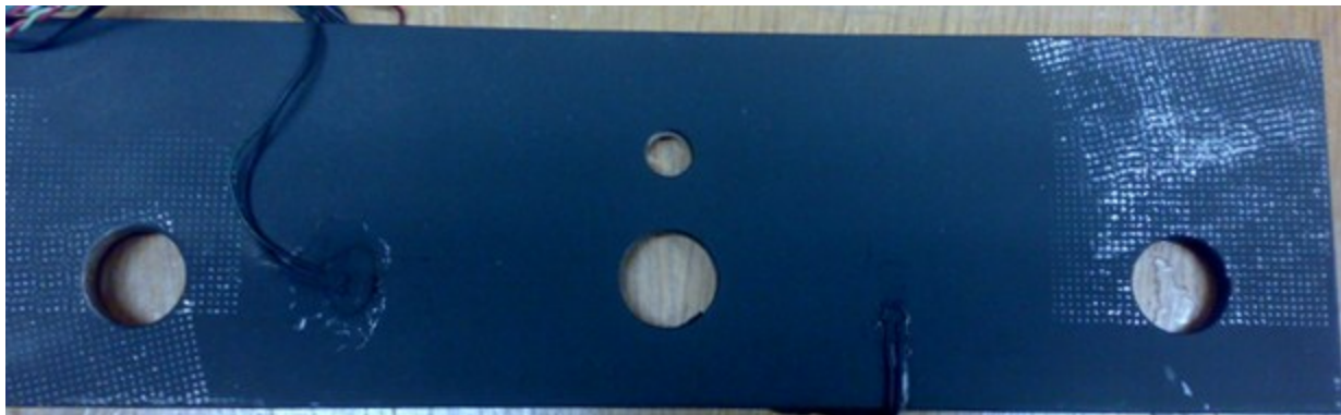
Fig. 8.3: Aluminum plate coated with Krylon Ultra-Flat black paint
