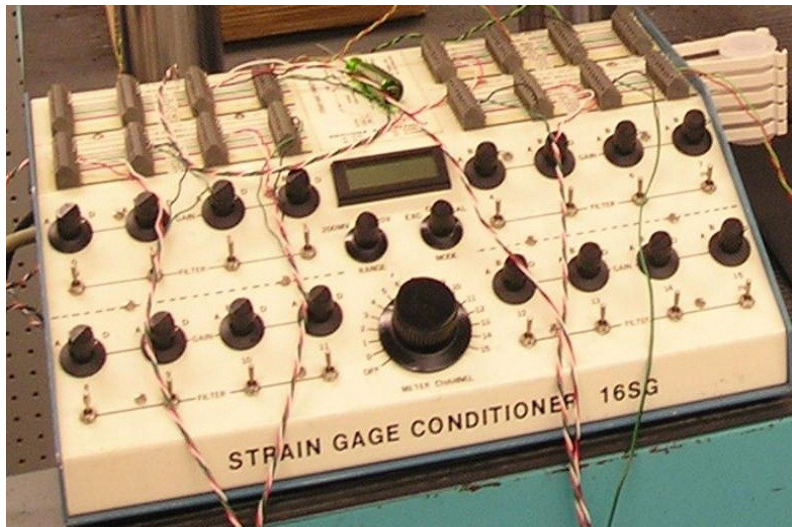
Fig. 8.94: 16 Channel, variable excitation strain gage conditioner
