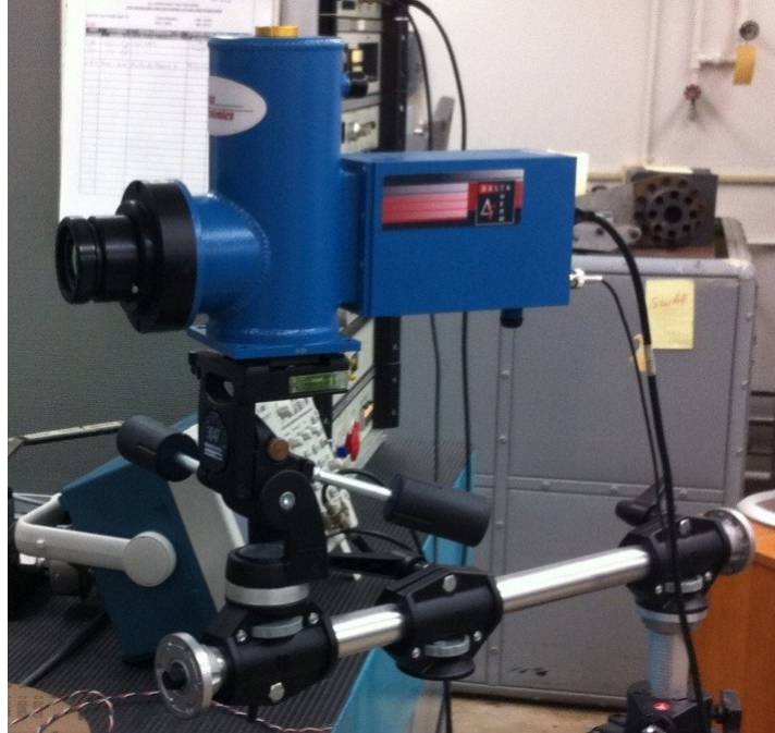
Fig. 6.18: TSA Delta Therm camera
