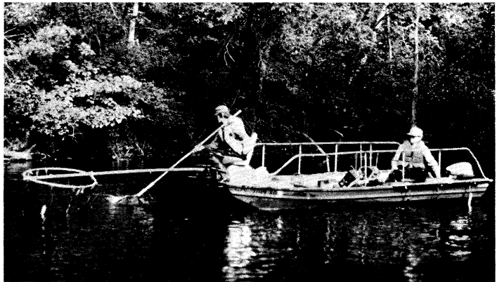
E. DC minishocker consisting of a 16-ft flatbottom aluminum boat, a 5-hp 240-volt DC generator, and a pulser control box. It is shown being used in the Apple River with Rick Tollefson dipping and David Siegler steering.
