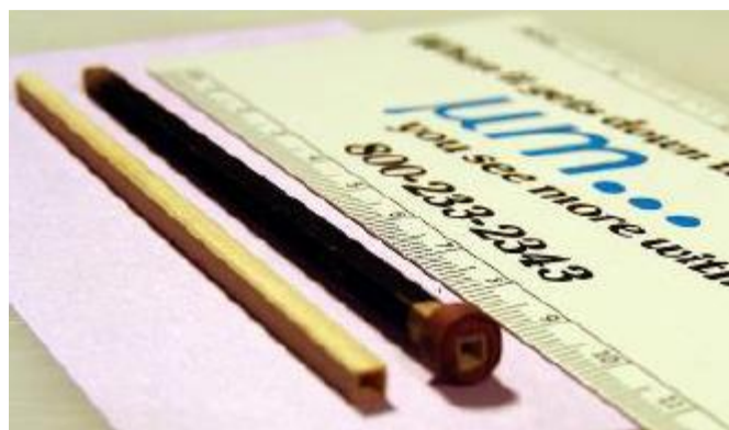
Figure 5-16: A Single channel sample cut from a filter [165]
