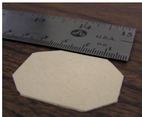
Figure 5-27: A cordierite wafer sample used in a full scale of particulate filter [168]
