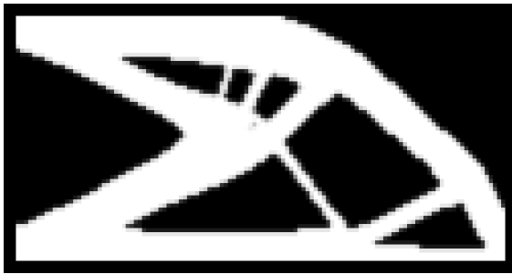
(a) Density distribution by SIMP with penalty factor equals 3.
