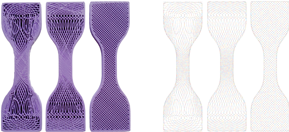
Figure 5.5: The FDM printed tensile test specimens. Left: from left to right, infill pattern A, infill pattern B and linear infill pattern. Right: the G-codes for the first two layers. Images of printed parts courtesy of [140].
