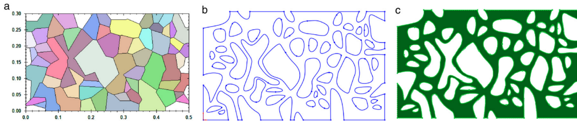
Figure 2.4: A procedural porous structure model. (a) The control polygons used for B-Spline curve fitting. (b) The pore geometries represented by B-Spline curves. (c) Boolean subtraction of the pores from the external geometry and the resultant 2D representation of the irregular porous structure. Image courtesy of [66].
