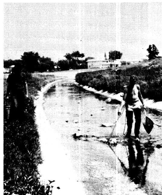
Underwood Creek (Milwaukee River basin) at end of 106 Street in City of Milwaukee. This concrete-lined creek is being sampled with a Tiny Tiger pack shocker.
