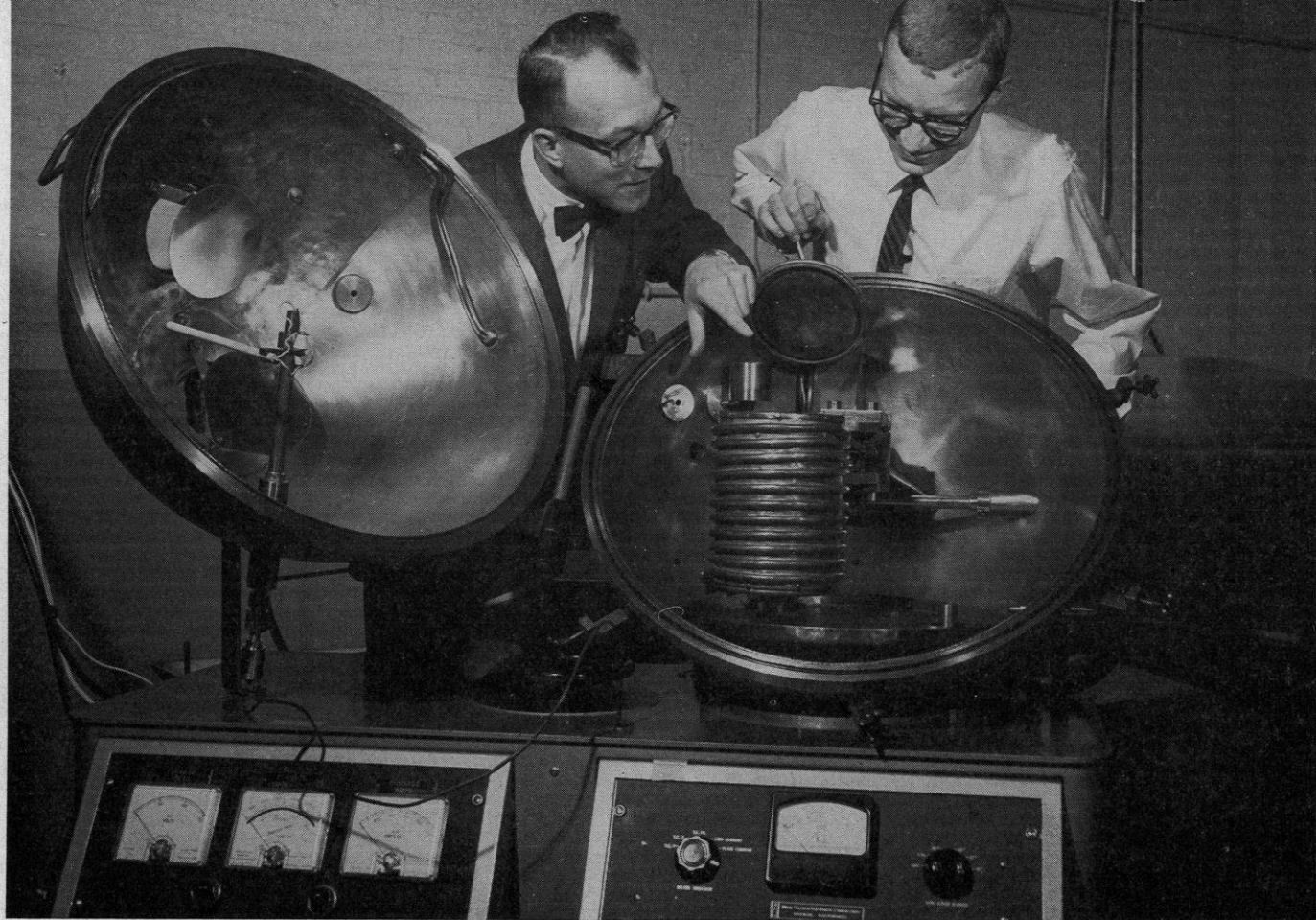
Prof. Franz Vitovec (left) and research assistant Brian Bagley, check a furnace used for melting or heat-treating such reactive metals as uranium and zirconium. The metals are used for study and research in the University's nuclear engineering program.
