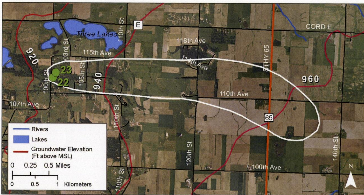
Estimated recharge area for spring #23. The discharge from this spring was 1.4 cfs, and the estimated recharge area was 2.1 mi 2 .
