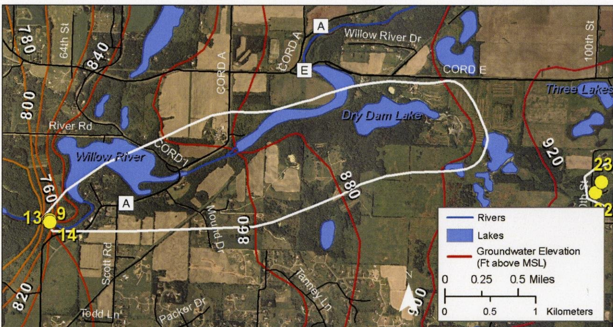
Estimated recharge area for springs #9 and #14. The discharge from these springs was 1.8 cfs, and the estimated recharge area was 1.9 mi 2 .
