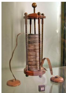
Figure A.2.1. Historical Voltaic pile (Como, Italy) made by A. Volta circa 1799.
