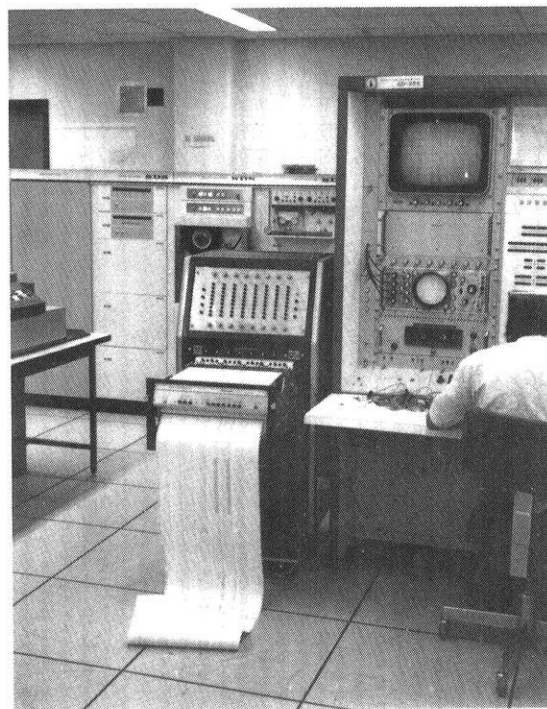
Eight channel strip recorder shows output from cardiovascular project.
