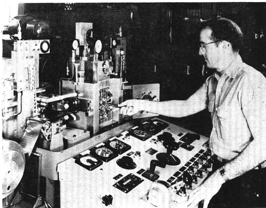
Rolling extra-thin, precision gage metal strip on specially designed Sendzimir mills at Hamilton Watch Company's Allied Products Division. Elaborate electronic and hydraulic controls on these mills permit continuous adjustment of strip tension and rolling pressure, thus make it possible to roll strip as fine as .00012-inch with thickness held to a tolerance of .00005-inch.
