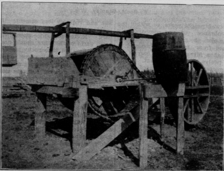
Mr. Scott's concrete mixer.
