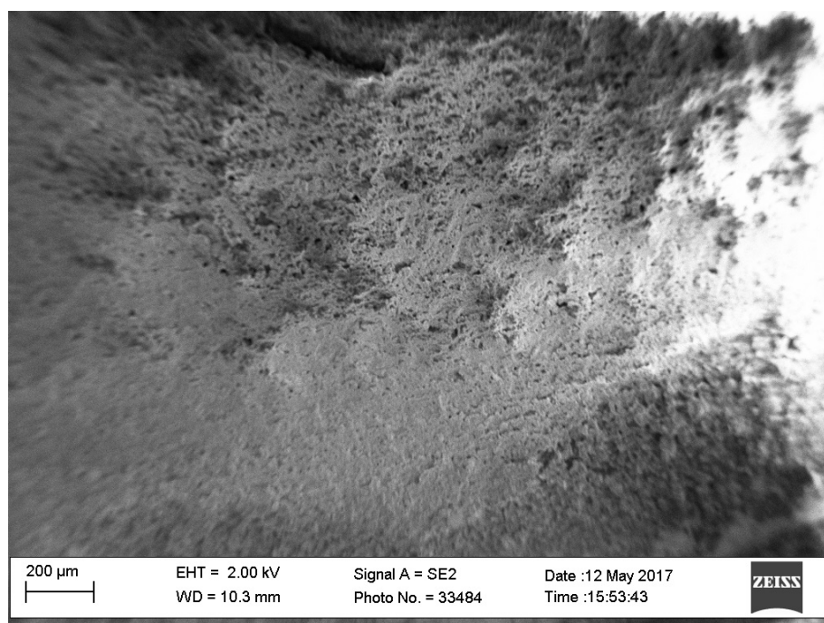
Figure A.49: SEM micrograph of Sn-MCM-41 deposited on ZnSe.
