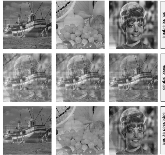
Figure C.2: Blind image signal separation using SCA. The three panel rows display three source images, three linear mixtures of the source images, and the three separated images using SCA.
