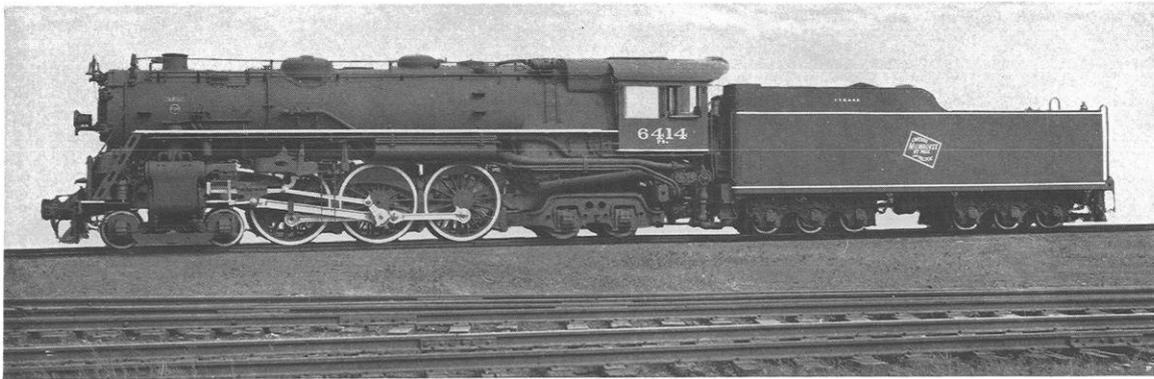
Upper: Early passenger locomotive. Lower: Modern passenger locomotive. Total weight 380,220 pounds. Diameter of drivers 72 inches. Wheel base 41 feet. Boiler pressure 225 pounds. Heating surface 4,200 square feet. Built 1931. Courtesy of the Baldwin Locomotive Works
