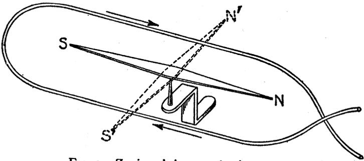
FIG. 2. Zweigger's improved galvanometer
