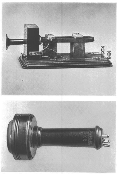
Upper: Bell's box telephone of 1877 with hammer called "Watson's thumper" used to attract the listener. Lower: Hand telephone receiver of 1877
