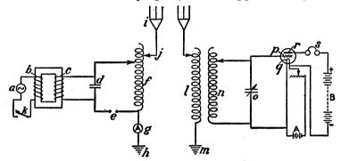
FIG. 30. A discontinuous-wave radio set
