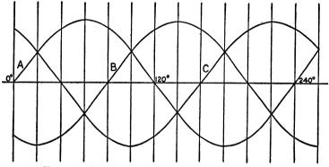
FIG. 14. Three-phase alternating current diagram
