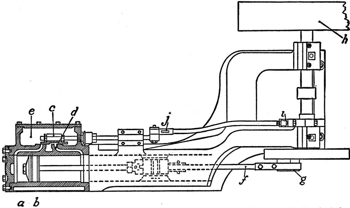
FIG. 33. Diagram of simple reciprocating steam engine. From Lieut. Col. W. A. Mitchell's "Mechanical Engineering." By permission of the author and John Wiley & Sons, Inc., publishers
