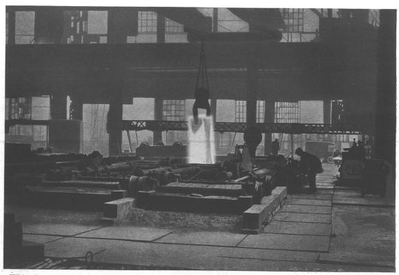
White-hot steel ingot being drawn from the soaking pit. Courtesy of the United States Steel Corporation
