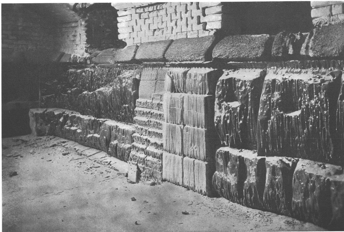
Differences between refractories in withstanding hot glass action. The Fulcher electrocast mullite blocks occupy the center of the furnace wall. Courtesy of the Corning Glass Works
