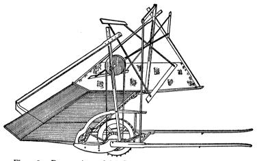
Fig. 58. Restoration of McCormick reaper, 1834. Drawing from patent specifications of C. H. McCormick, omitting the pusher device
