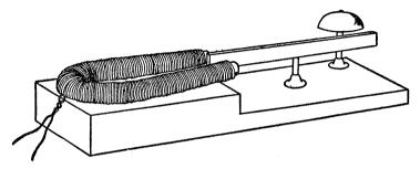
FIG. 20. Henry's electromagnetic telegraph operated at Albany, N. Y., as early as 1831, through a mile of line wire
