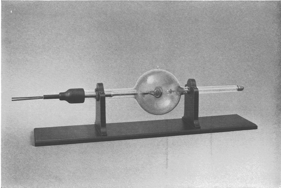
Modern Coolidge X-ray tube. Courtesy of the General Electric Company
