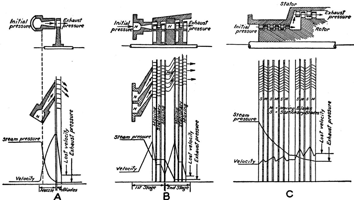
FIG. 34. A. Diagram of De Laval steam turbine. B. Diagram of Curtis steam turbine. C. Diagram of Parsons steam turbine. From Lieut. Col. W. A. Mitchell's "Mechanical Engineering." By permission of the author and John Wiley & Sons, Inc., publishers
