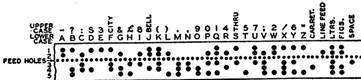
FIG. 24. A code-punched paper ribbon used in the modern printing telegraph
