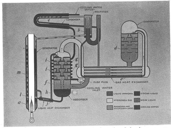
Domestic absorption refrigerator. Operates by transfer of ammonia gas by heat from strong water solution, cooling and expanding. Courtesy of the Electrolux Refrigerator Sales, Inc.
