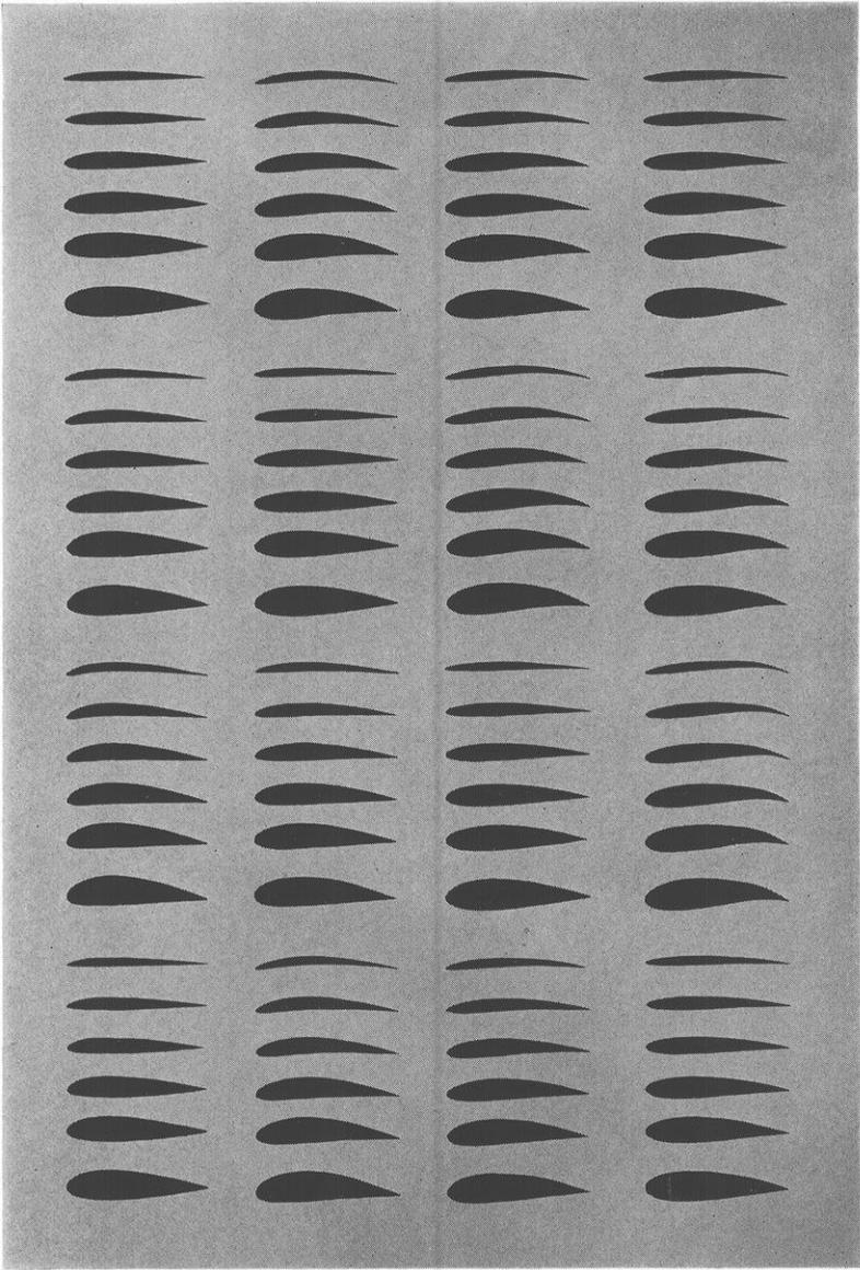
AN EXAMPLE OF THE VARIETY OF AIRFOIL SECTION SHAPES INVESTIGATED IN THE N.A.C.A. VARIABLE-DENSITY WIND TUNNEL
