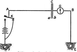
FIG. 25. Cable operation through electric condenser
