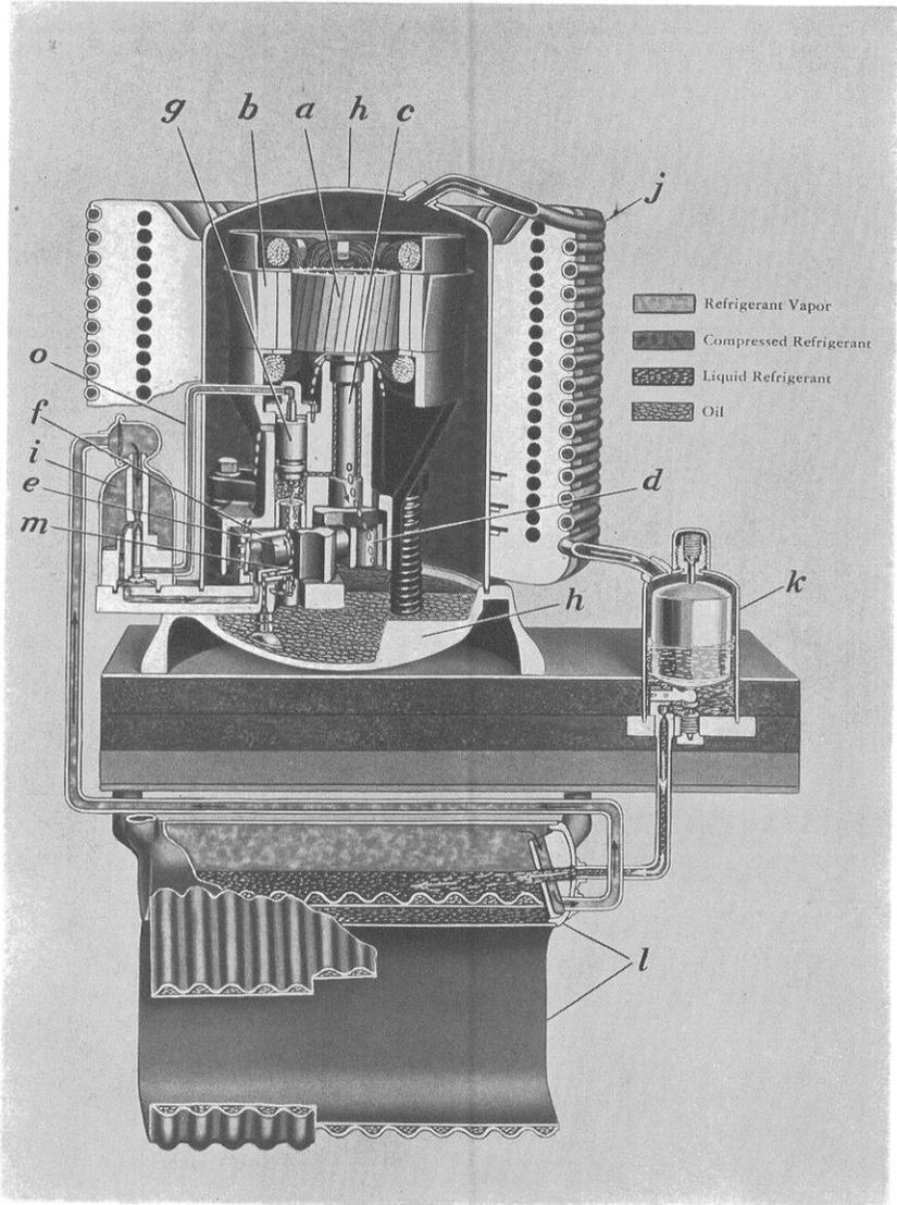
Domestic compression refrigerator. Operates by highly compressing sulphur dioxide gas, cooling and expanding. Courtesy of the General Electric Company
