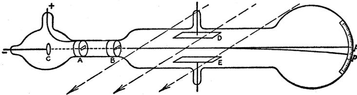
FIG. 16. J. J. Thomson's discovery of the electron. Cathode rays, which are electrons in motion, tending to be deflected to  $p'$  by the magnetic field indicated by the arrows, are restored to  $p$  by the electric field,  $DE$ . From the electric and magnetic quantities involved, Thomson determined the charge and mass of the electron
