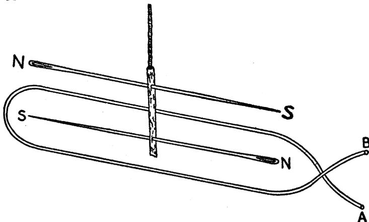
FIG. 3. Faraday's galvanometer
