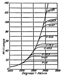
FIG. 17. Cathode temperature, voltage, and thermionic current. The strength of thermionic current soon reaches a maximum for any given voltage, owing to space charge. After Langmuir
