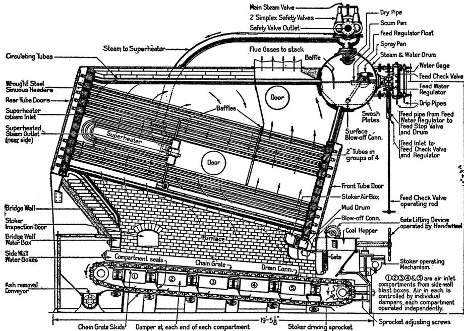
FIG. 32. Babcock and Wilcox tubular boiler; from S.S. *City of Saginaw*. Typical installation of 1929. Chain grate stoker, 5,190 square feet boiler surface, 315 pounds working steam pressure
