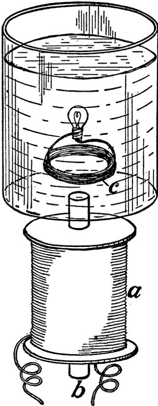
FIG. 12. Experiment illustrating electric repulsion
