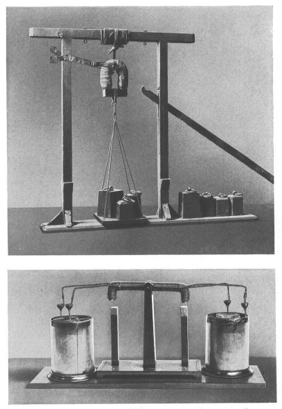
Upper: Henry's Yale magnet, which supported 2,063 pounds. Lower: Henry's electromagnetic oscillating motor
