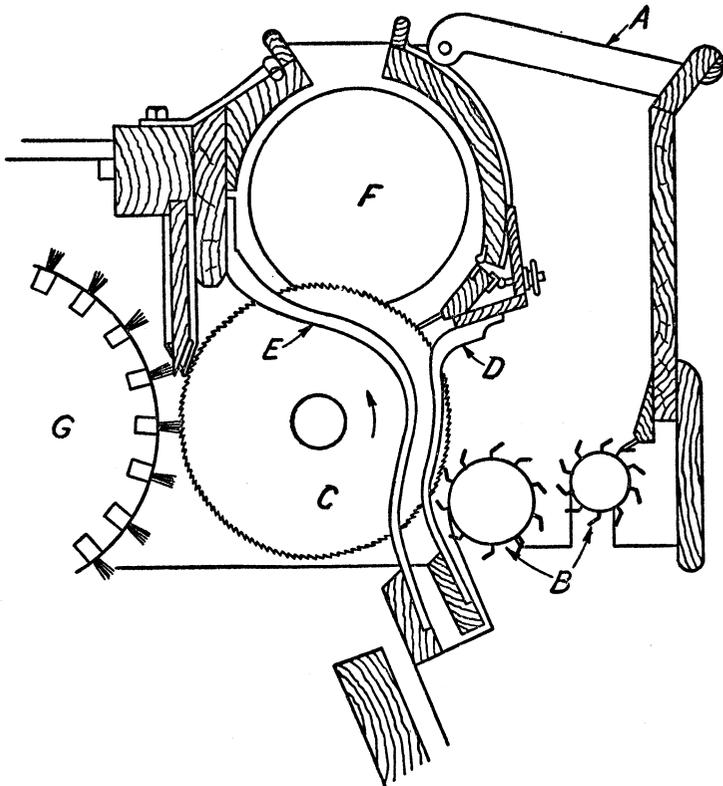
FIG. 57. Cross sectional diagram of a cotton gin. Courtesy of John Wiley & Sons, Inc., publishers
