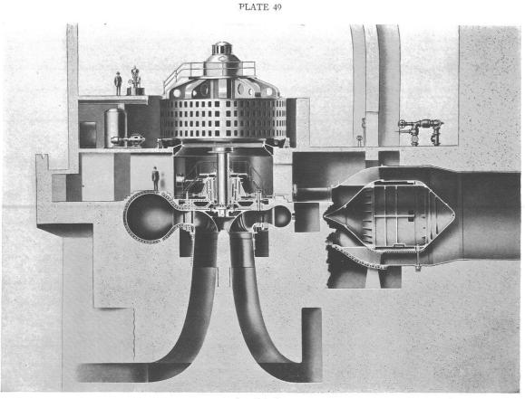
Niagara Falls. Sectional view of 70,000 h.p. turbine. Courtesy of the Niagara Falls Power Company
