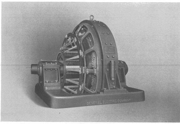
Direct-current motor, 14 pole, 2,600 h.p. Courtesy of the General Electric Company
