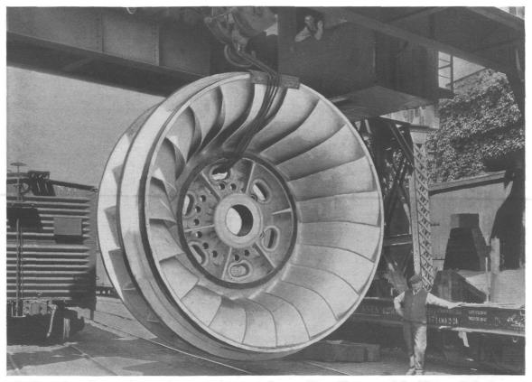
Single steel casting, 52½ tons, the runner for 70,000 h.p. turbine. Courtesy of the Niagara Falls Power Company
