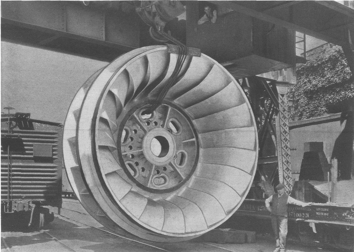
Single steel casting,  $52\frac{1}{2}$  tons, the runner for 70,000 h.p. turbine. Courtesy of the Niagara Falls Power Company
