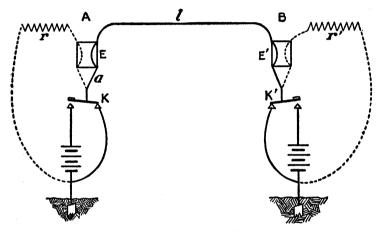
FIG. 23. Duplex telegraph diagram
