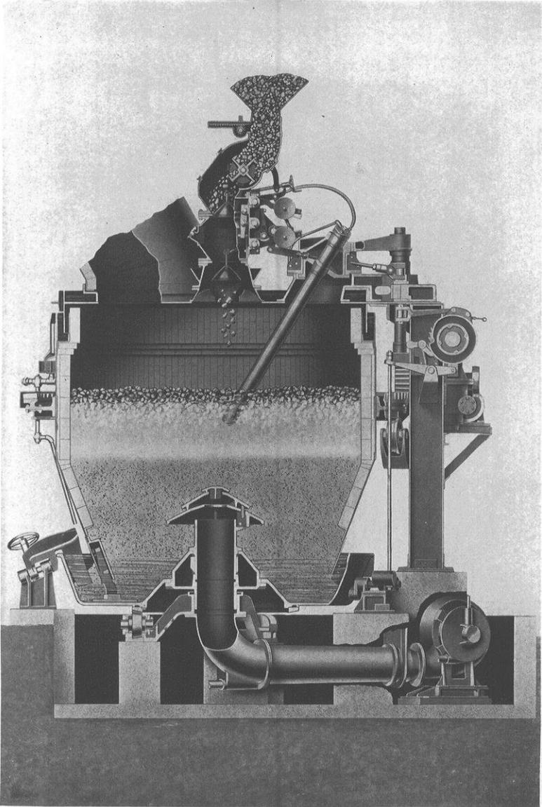
Vertical section of Wellman producer gas plant. Courtesy of the Wellman Engineering Company
