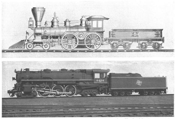
Upper: Early passenger locomotive. Lower: Modern passenger locomotive. Total weight 380,220 pounds. Diameter of drivers 72 inches. Wheel base 41 feet. Boiler pressure 225 pounds. Heating surface 4,200 square feet. Built 1931. Courtesy of the Baldwin Locomotive Works
