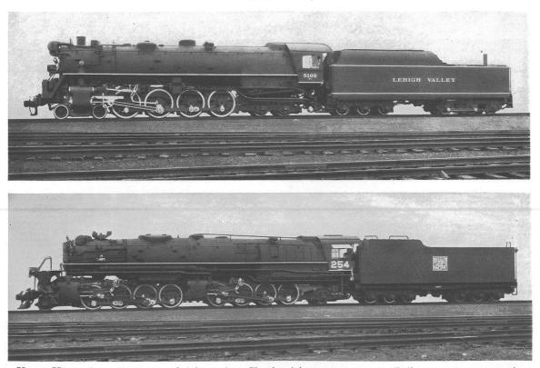
Upper: Heavy-duty passenger or freight engine. Total weight 408,000 pounds. Boiler pressure 250 pounds. Heating surface 5,422 square feet. Tractive force 66,400 pounds. Built 1931. Lower: Articulated locomotive for heavy freight duty. Total weight 665,100 pounds. Tractive force 137,000 pounds. Courtesy of the Baldwin Locomotive Works
