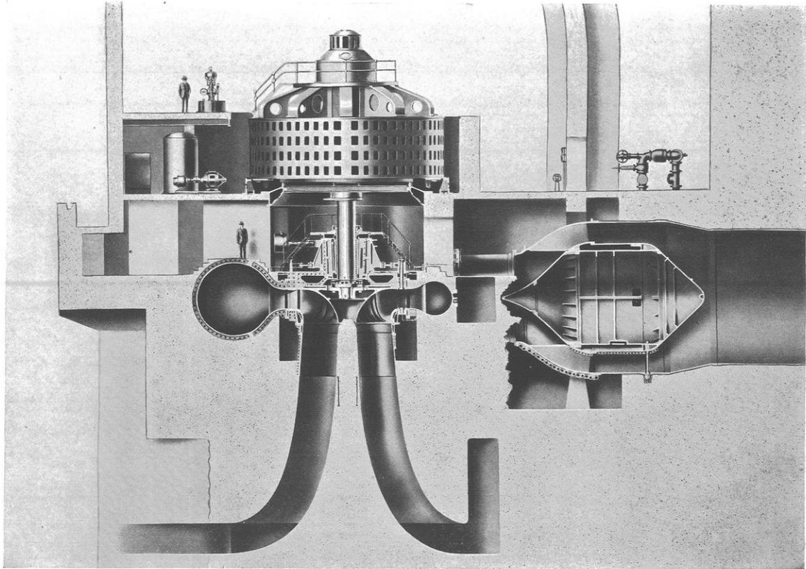
Niagara Falls. Sectional view of 70,000 h.p. turbine. Courtesy of the Niagara Falls Power Company
