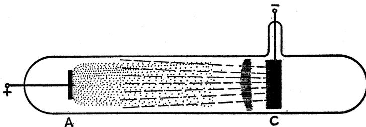
Fig. 15. Electric discharge in a high vacuum (diagrammatic)
