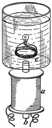
FIG. 12. Experiment illustrating electric repulsion
