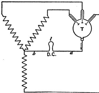
FIG. 19. Cooper Hewitt mercury rectifier. Three-phase alternating current connected to three iron electrodes in glass bulb, *T*. When any one of them becomes positive the current flows to the mercury electrode at the bottom, and passes as a direct current from *a* to *b* through circuit, *I*.
