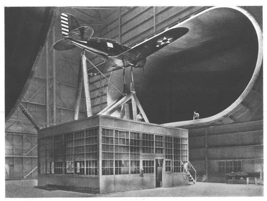
TEST CHAMBER OF THE N.A.C.A. FULL-SCALE WIND TUNNEL A modern military airplane with cowled radial engine and retractable landing gear is mounted on the balance for test
