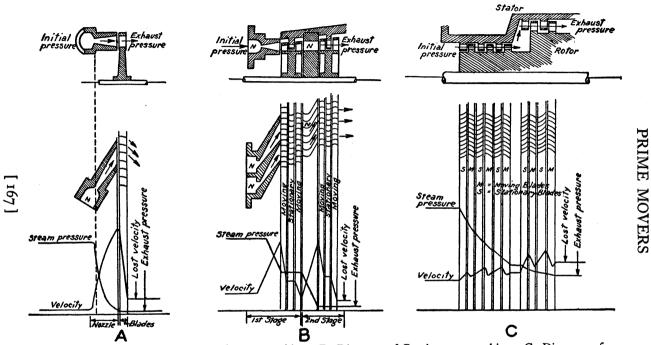
FIG. 34. A. Diagram of De Laval steam turbine. B. Diagram of Curtis steam turbine. C. Diagram of Parsons steam turbine. From Lieut. Col. W. A. Mitchell's "Mechanical Engineering." By permission of the author and John Wiley & Sons, Inc., publishers
