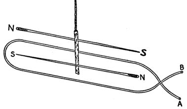
FIG. 3. Faraday's galvanometer
