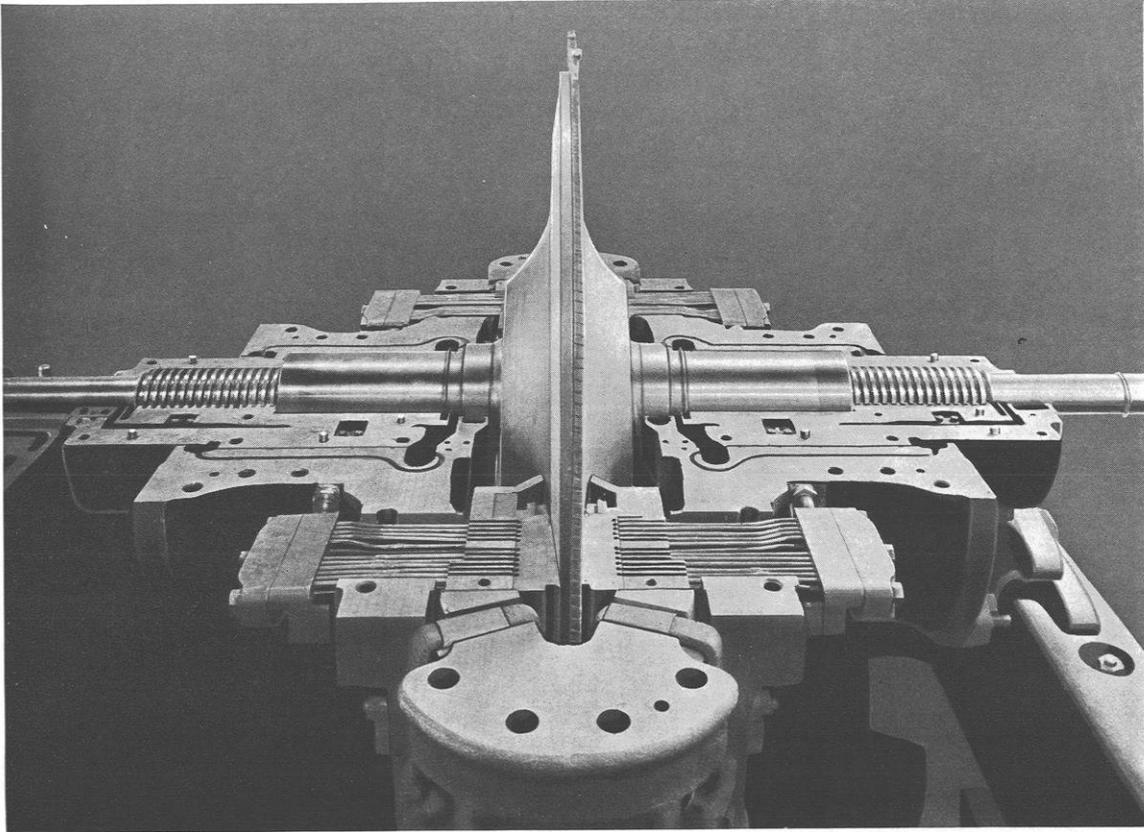
Alexanderson high-frequency dynamo for radio transmission. Top removed to show details. Courtesy of the General Electric Company
