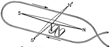
FIG. 2. Zweigger's improved galvanometer
