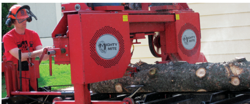
Nothing goes to waste. Evergreens removed from the Badger School site were sawed into boards (below) on-site with a portable sawmill. The lumber will provide boards for benches. Smaller twigs and residues will be chipped into mulch.
