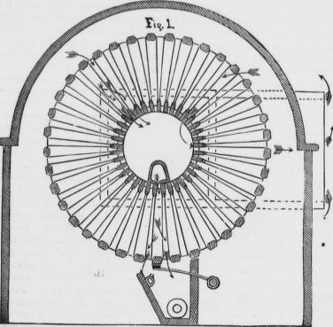
to it. As the section that is being cleaned fans of purifiers blowing, while the fan on dust collector is sucking the air through. It is understood that the principle of our dust collector is that of drawing through and not blowing in. However, by the above mentioned operation, the results accomplished are the same.
