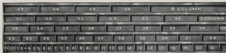
No. 5446 Unit. Length, 52 inches. For labor-saving column rules—divisions from 2 to 50-pica ems by ems, varying by half picas from 1 to 9 \frac{1}{2} ems, also compartments for 1, 3 and 8-column rules.
