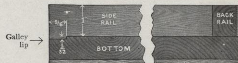
Showing the construction of the job letterboard with back rail and lip at the front to receive the galley.
