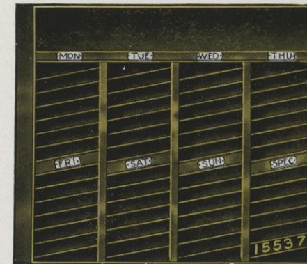
Unit 15537 Holds 48 Double-Col. Galleys for Overrun Ads Width, 33\frac{3}{4} inches
