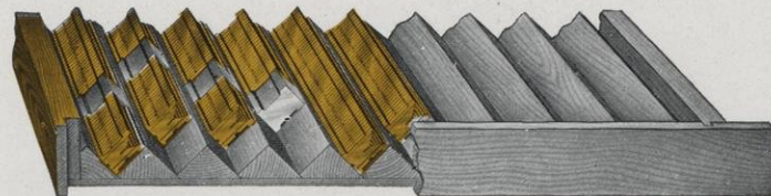
Detailed Section of Matrix Drawer, showing Matrices in place
