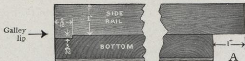
Showing the construction of the newspaper letterboard. This letterboard has no back rail. The side rails extend one inch (A), acting as supports when type forms are transferred to cast-iron imposing surfaces.
